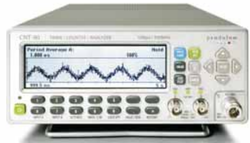
Figure 5: Display showing the trend (signal over time) of sampled data.
